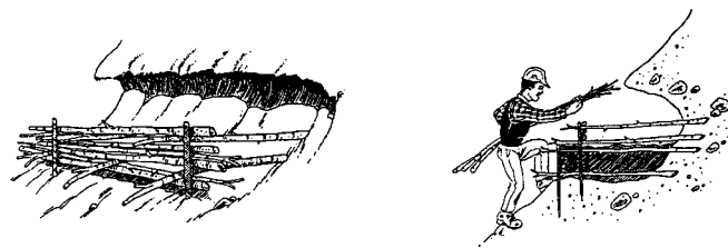
Figure 10. Live reinforced earth walls are constructed with a wattle fence on the face and long cuttings going back into the slope to hold the face in place. Re-sloping the overhang provides the backfill while the LaREW provides a vegetated cover on the undercut area.
