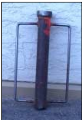
Figure 3. Specialized rebar pounding tool made out of pipe and bars.
