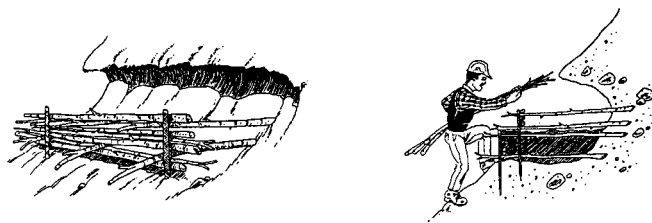
Figure 10. Live reinforced earth walls are constructed with a wattle fence on the face and long cuttings going back into the slope to hold the face in place. Re-sloping the overhang provides the backfill while the LaREW provides a vegetated cover on the undercut area.
